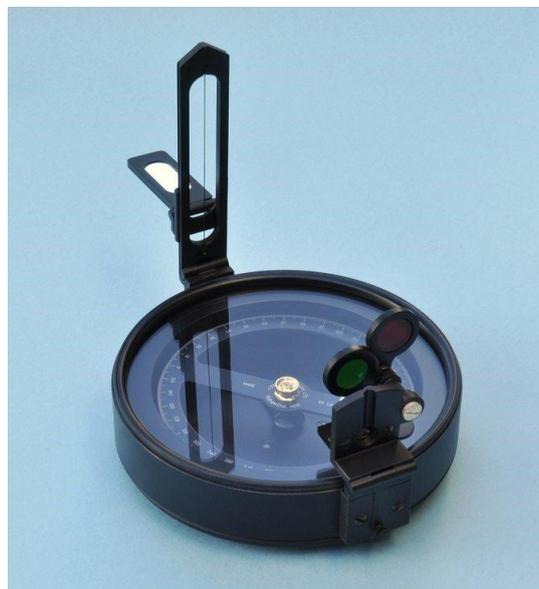
Compass surveying is not used in places which contain iron core, power lines etc which usually attracts magnets due to their natural properties and electromagnetic properties respectively. Compass surveying is done by using traversing. A traverse is formed by connecting the points in the plot by means of a series of straight lines.
