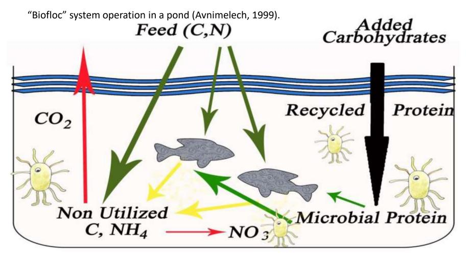
Biofloc technology is a system that has a self-nutrification process within culture pond water with zero water exchange (Yoram, 2012)
