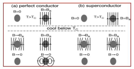
Figure 5 (a): Behaviour of a 'perfect conductor', i.e. a material which merely has zero resistivity below  $T_c$  (b): situation for a genuine superconductor which displays the Meissner effect.
