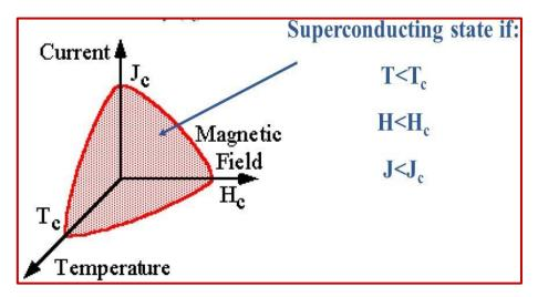
Figure 7: Schematic of the regions of current density, magnetic field and temperature within which a material remains superconducting
