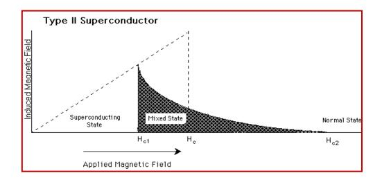
Figure 9: Induced magnetic field versus applied magnetic field of a Type II superconductor.
