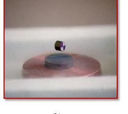
**(b)** Figure 4: (a) Meissner effect with magnetic field lines (represented as arrows) excluded from a superconductor when cooled below its critical temperature. (b) A
