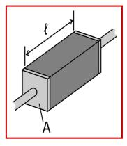
Figure 2: A piece of resistive material with electrical contacts on both ends.
