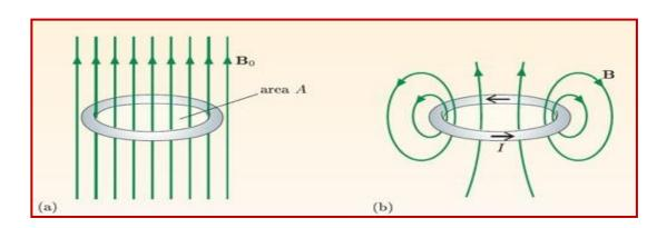
Figure 1: (a) A superconductor in magnetic field (b) Persistent current flowing in superconductor after the removal of field.
