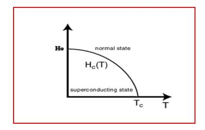
Figure 6: Effect of magnetic field and temperature on a superconductor.
