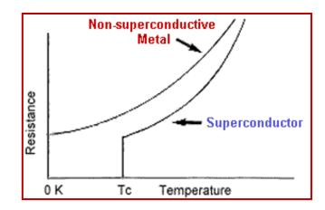
Figure 3: Variation of resistance of metals with temperature
