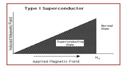
Figure 8: Induced magnetic field versus applied magnetic field of a Type I superconductor.
