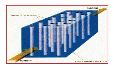
Figure 10: A current-carrying type II superconductor in the mixed state showing magnetic vortices
