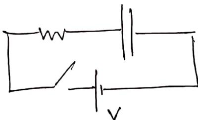
Let steady potential 'V' applied to circ., 'i' be instantaneous value of current through 'R', potential at the plane of condenser will be
