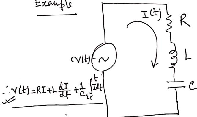
$V(t)$  is connected in series with resistance ' $R$ ', inductance ' $L$ ' and capacitance ' $C$ '
