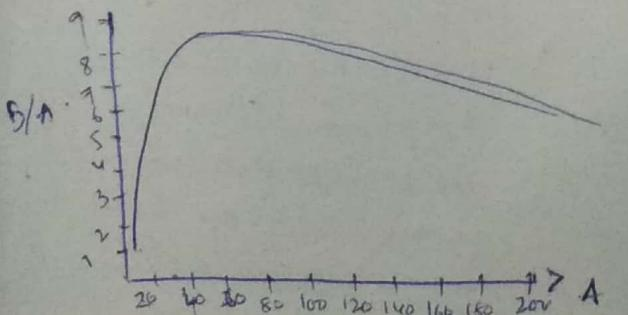
The decrease of  $\frac{B}{A}$  for large  $A$  is due to Coulomb repulsion between the protons which make the nuclei less stable.
