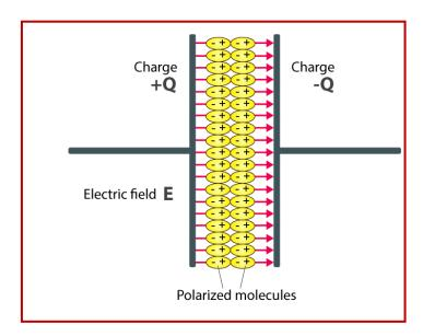
Figure 1: Polarisation of dielectric molecules when the electric field is applied.
