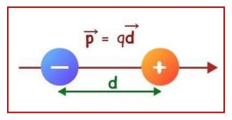
Figure 2: Electric dipole moment
