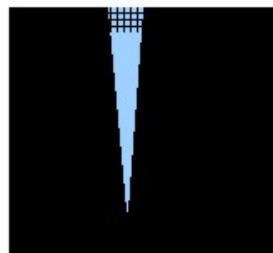
A small crack in a rock fills with water during the daytime. As the water begins to freeze at night, it starts at the top, sealing the crack.
