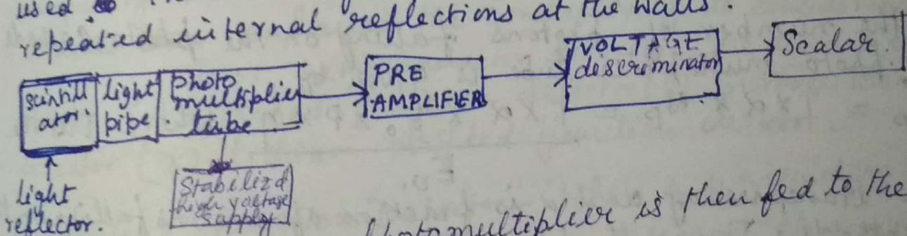
The output from a photomultiplier is then fed to the amplifier, scalar and recorder.
