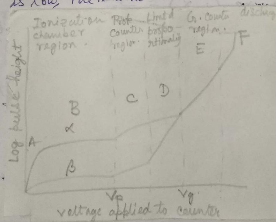
This is the region of Ionization chamber. As the voltage is increased gradually the secondary ionization by collision or the avalanche ionization takes place in the region where the electric field is very high i.e. near the central wire.
