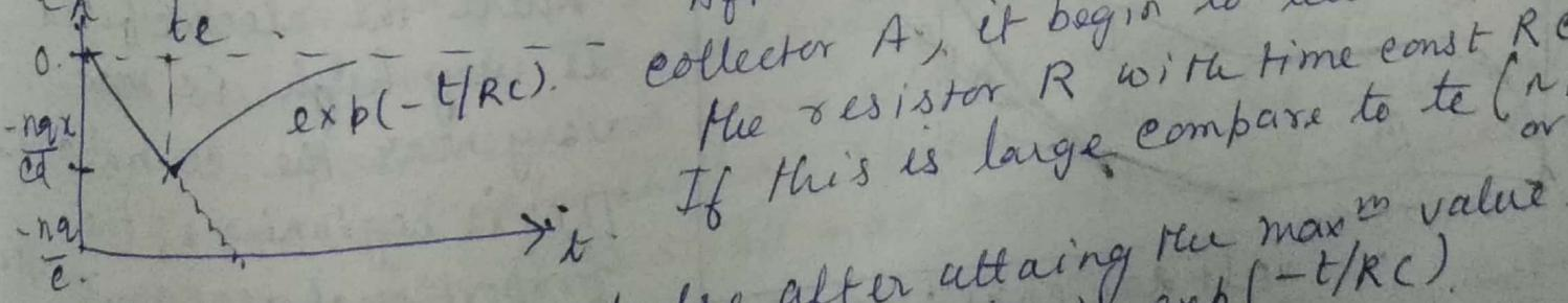
Then the voltage pulse after attaining the max<sup>m</sup> value falls off exponentially.  $v_C = (v_e) \cdot \exp(-t/RC)$ .
