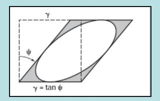
In **homogeneous** strain, two orientations of material lines remain perpendicular before and after strain. These two material lines form the axes of an ellipse that is called the **strain ellipse**.
