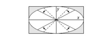
Homogeneous strain describes the transformation of a square to a rectangle or a circle to an ellipse. Two material lines that remain perpendicular before and after strain are the principal axes of the strain ellipse (solid lines).
