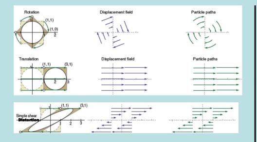
Translation moves every particle in the rock in the same direction and the same distance, and its displacement field consists of parallel vectors of equal length.
